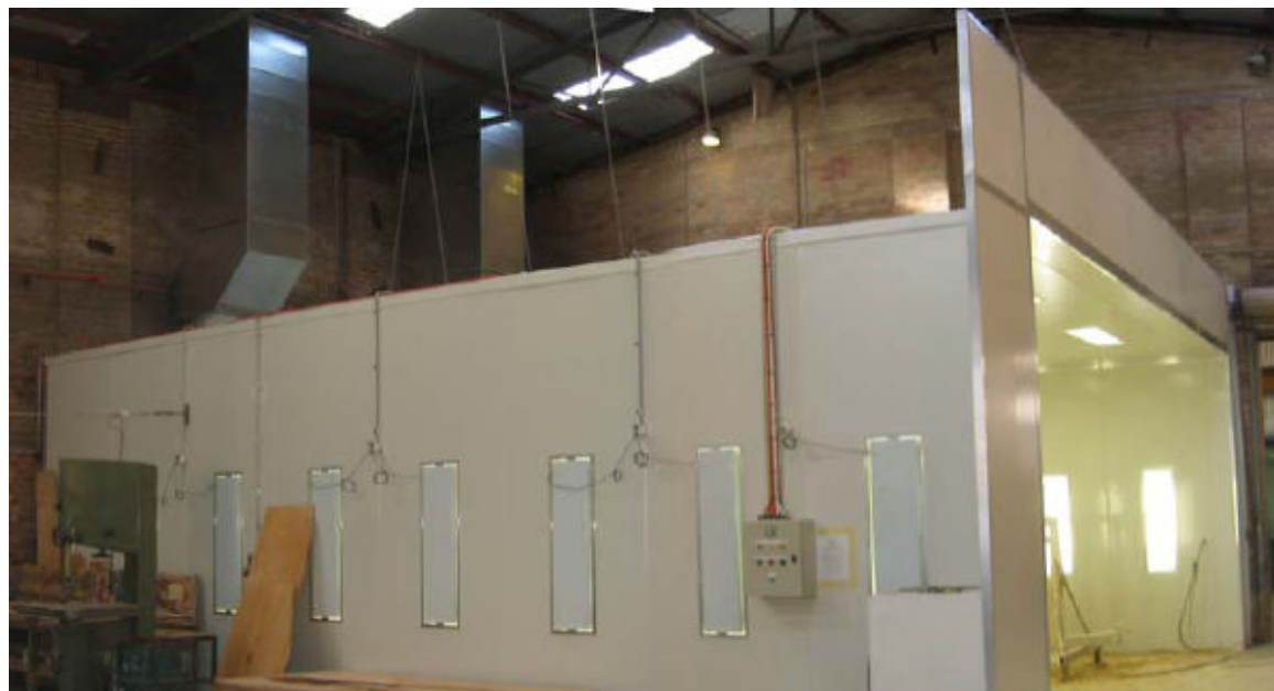
The 10S Cabin has a High Visibility Cabin with Rear Access Lighting
